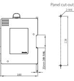
Mounting Mounting on DIN rail with bolts
